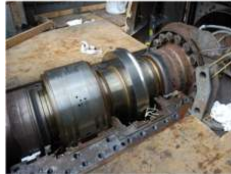
Thrust Bearing at 7 Years of Operation with the ISOPur purification Unit
